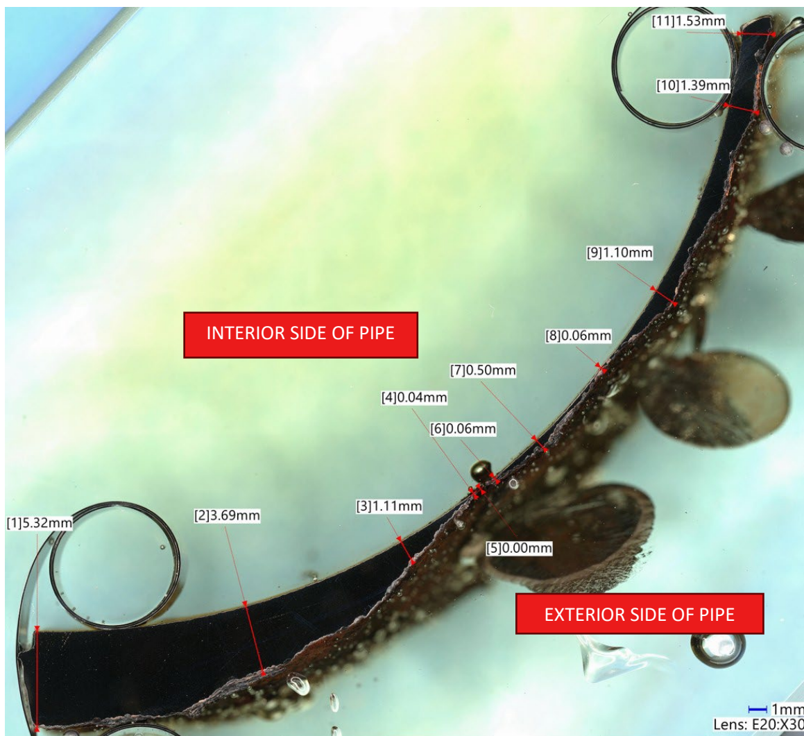
Figure 21: The pipe wall was found to be thinned in the area of the two holes.
